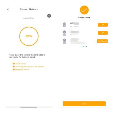
Note: When adding the camera, ensure the WIFI network is good, the camera is normally turned on, and the indicator light flashes red slowly. After the connection is successful, the indicator light is blue.
