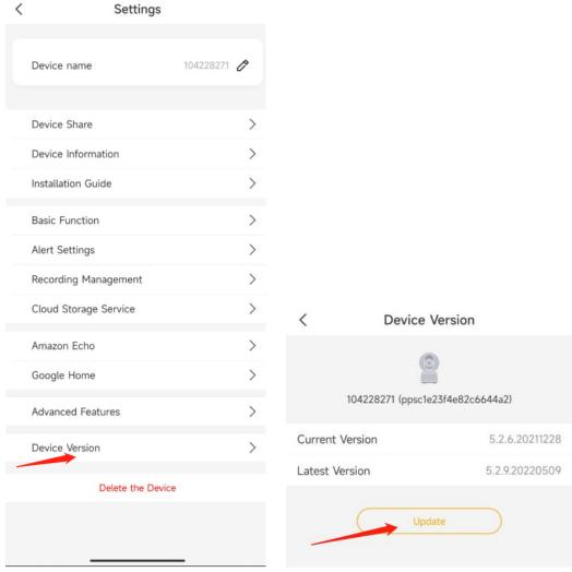
If have new firmware to be upgraded, you can tap 'upgrade' to upgrade the camera firmware.
